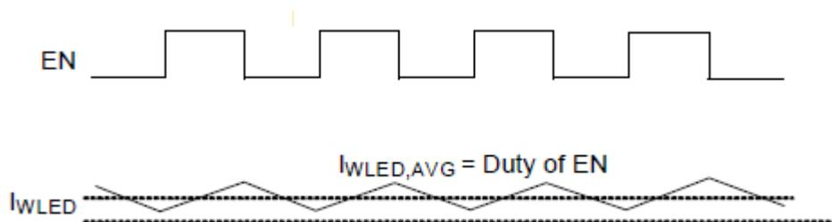
Figure 1. PWM Dimming
