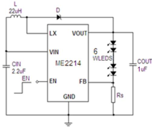
$I_{LED} = 20\text{mA}$ ,  $R_s = 10\Omega$
