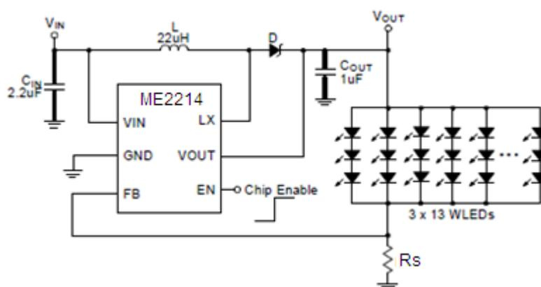
Figure 5. Application for Driving 3 X 13WLEDs
