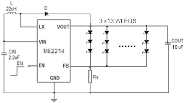
$I_{LED} = 260\text{mA}$ ,  $R_s = 0.77\Omega$
