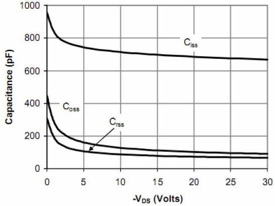
Figure 8: Capacitance Characteristics
