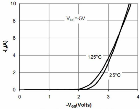
Figure 2: Transfer Characteristics
