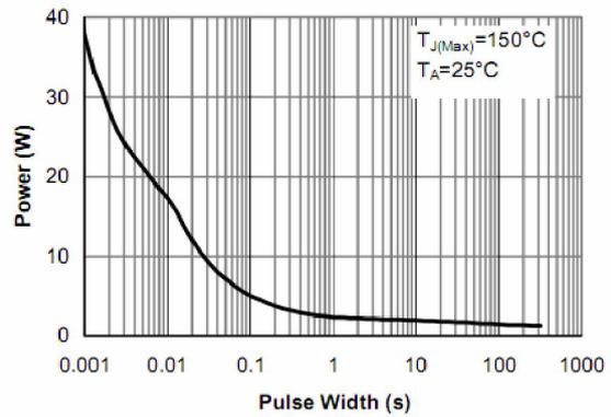
Figure 10: Single Pulse Power Rating Junction-to-Ambient (Note E)
